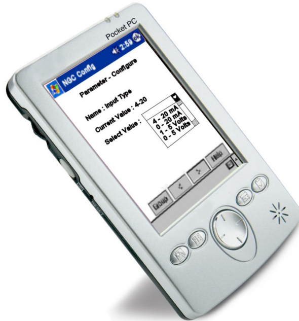
Pocket PC running Process Instrument Explorer
