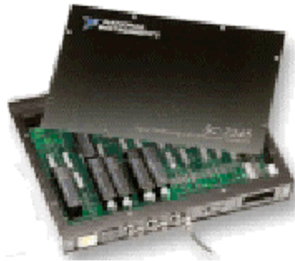
SCC Series signal conditioning with sensors and TEDS interfaces
